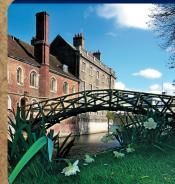
This, the only wooden bridge spanning the River Cam, was first built in 1749, to a design by the civil engineer, William Etheridge. The original bridge was made from oak, but the structure you see today is a teak-built replica from 1904. Contrary to popular legend, the bridge has always had iron bolts at the joints.
